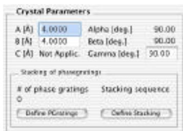
Only A and B and Gamma have meaning for a layered “structure”. The buttons “Define PGratings” and “Define Stacking” are used to choose the different projected potentials and to define their sequence to make up the entire specimen.
