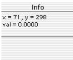
This window shows the current position of the cursor within the image window and the intensity of the underlying pixel. When dragging a rectangle, the dimensions of the rectangle are shown. Line lengths and angles are also displayed. Image statistics is displayed in this window when invoked through the “Statistics” in the “Process” menu.
