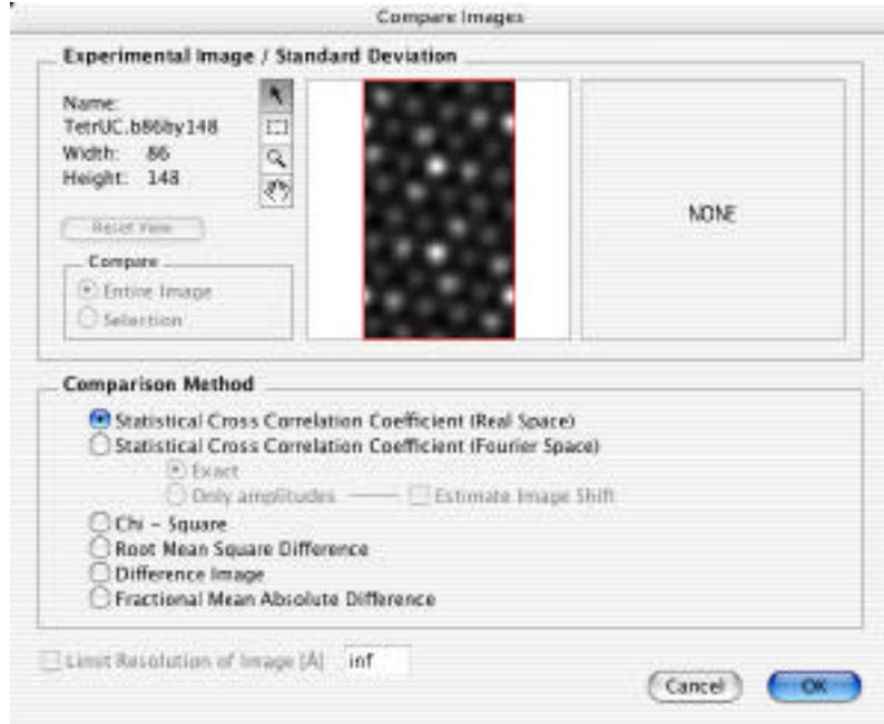
When comparing images, the experimental image will be resampled such that the sampling corresponds to the sampling of the calculated image.
