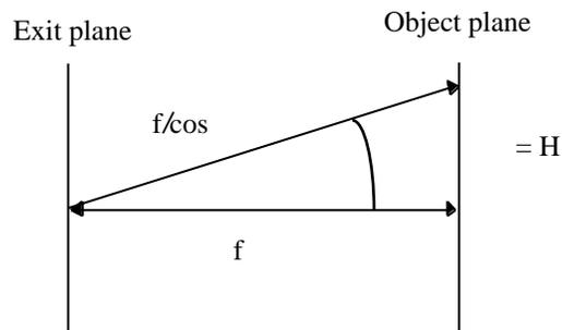
The electron traveling along the optic axis will have a path length of  $f$  while an electron that has been scattered an angle  $=H$ , will travel a distance  $f/\cos$ . This can be expressed as a phase difference
