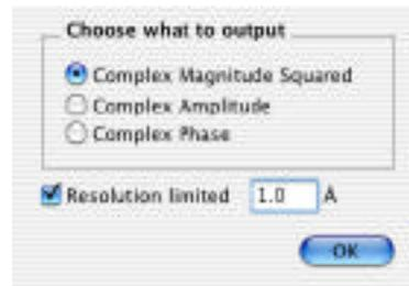
(magnitude squared, default), or if the image plane wavefunction(s) has been calculated, the complex amplitude or the complex phase of the electron wavefunction at the image.
