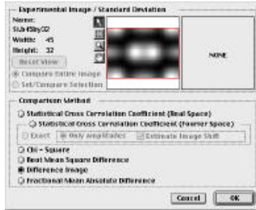
There are two calculations performed in this case. One gives a difference image(s) which are pseudo colored such that where the experiment and simulation agree within one standard deviation, the pixel is black, less than 1.5 standard deviations, the pixel is colored green, and outside the pixels are shown in
