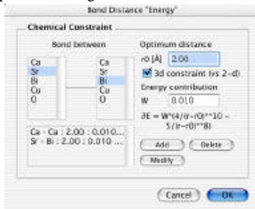
which can be used to specify a configuration energy that includes terms that depend on bond distances. It is possible to specify the optimum bond distance between two atoms, whether it is a 2d or 3d constraint, and to specify the weight of the term in the energy calculation. Even though bond distances have been defined, the inclusion of a bond-distance energy term can be turned off/on from the main “Refine Structure” window.
