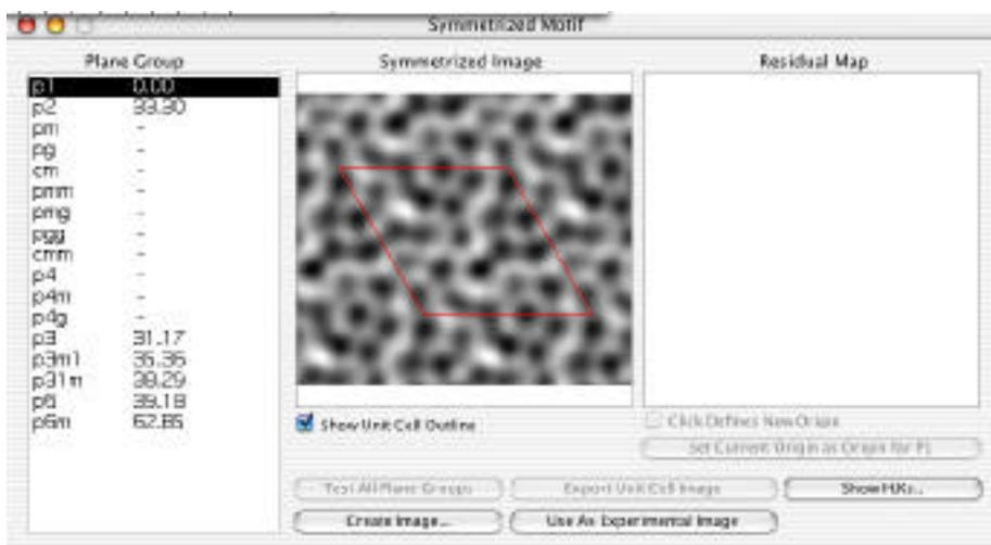
Each symmetry can be tested and imposed on the reflections to form a new unit cell motif. The origin of the unit cell motif is shown on the right and can be changed.
