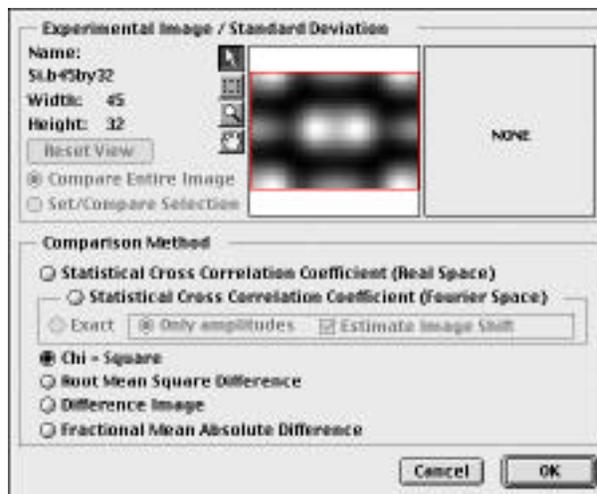
If no standard deviation image is given, the uncertainty in the pixel value is set to 10% of the intensity in the pixel. The Chi-square goodness of fit criteria is sensitive to the mean level of the images and the scales the calculated images so that they have the same mean as the experiment before computing chi-square. Lower values indicate better fit, with a value of 1 meaning that the experiment and simulation agree within the uncertainty of the experimental values.
