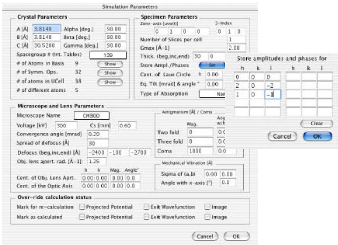
are determined by entering the hkl values for the reflection. Only 10 reflections can be tracked this way.
