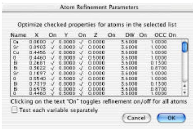
Normally varying the z-coordinate will not have any effect since the image simulation procedure uses a 2d projection of the atoms in the unit cell. However, in the case where symmetry operators are used, changing the z-position may result in changes in x and y for symmetry related atoms.
