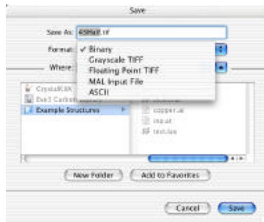
files are binary files used by the mal or TrueImage program for exit wave reconstruction from a through focal series.
