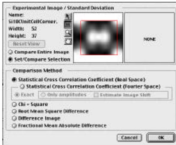
This is a straight calculation of the normalized cross correlation coefficient between the experiment and the calculated image(s). For it to give meaningful results, the origin of the experimental image needs to coincide with the calculated image.
