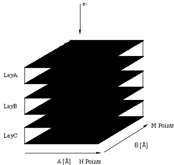
slices with different atomic content. As an example we will work with three layers which we will call LayA, LayB and LayC. Each of these “layers” are what we would call a “single” structure. That means they are defined as a unit cell with lattice parameters and atomic content. The one thing they have in common is that the lattice parameters A and B with respect to the electron beam are the same and that we will use identical sampling in each case, see figure above.
