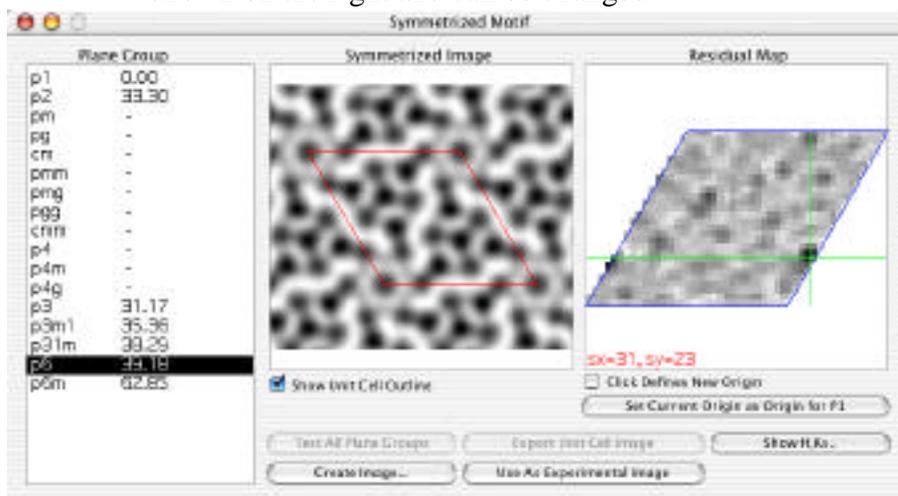
Once a solution has been chosen, a new image can be created with the imposed symmetry and can be used as an image to compare with simulation.
