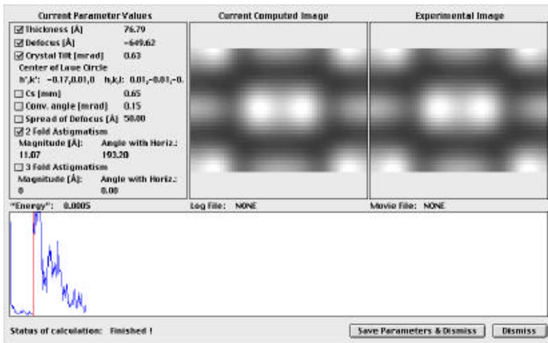
log file can be written so that the “energy” as a function of time/temperature can be plotted and also a Movie can be produced and played back. The number of frames/second for output can be set.
