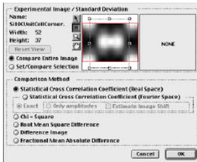
Note: The selection does not work for the Difference Image which automatically compares the entire image.
