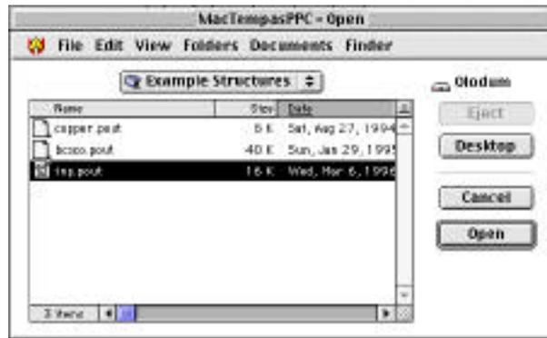
Double Click on LayA.pout and fill in the value for the slice-thickness that was used in the calculation of LayA.pout. Continue and do the same for LayB and LayC.
