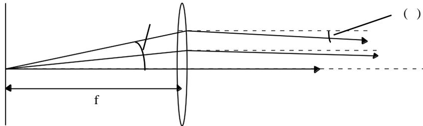
However, the spherical aberration of the lens causes a phase shift relative to the path of the unscattered electron ( $\alpha = 0$ ) which is written as (Scherzer, 1949):
