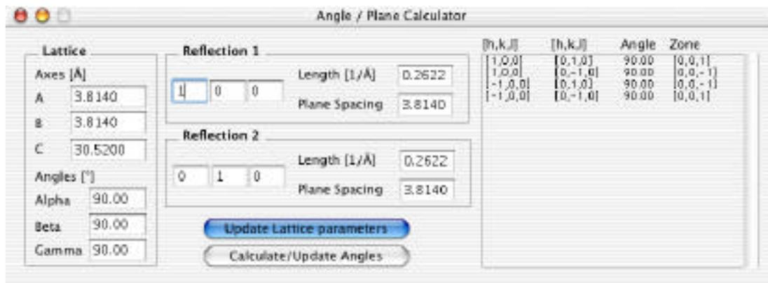
when the “Calculate?Update Angles” button is clicked, the angles between the family of reflections and the zone in which they occur will show to the right. The length of the vectors and the corresponding plane spacing is updated live when typing in a new reflection. The lattice parameters can be changed and invoked through the “Update Lattice Parameter” such that the calculator can be used for structures different from the one that is loaded.
