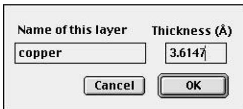
Now the program has information as to which phase-gratings it can use and the final part is to define the sequence of these phasegratings up to the desired thickness. Use “**Stack**” and the sequence can be defined in different ways. One way is to type
