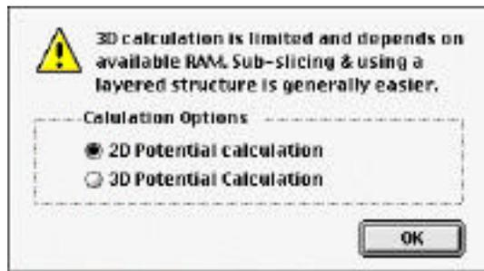
When a two-dimensional calculation is selected, MacTempas will use one slice per cell if the cell repeat distance in the beam direction is small. If the repeat distance is too large for one slice per unit cell, MacTempas will avoid pseudo-upper-layer-lines by producing  $n$  identical sub-slices.
