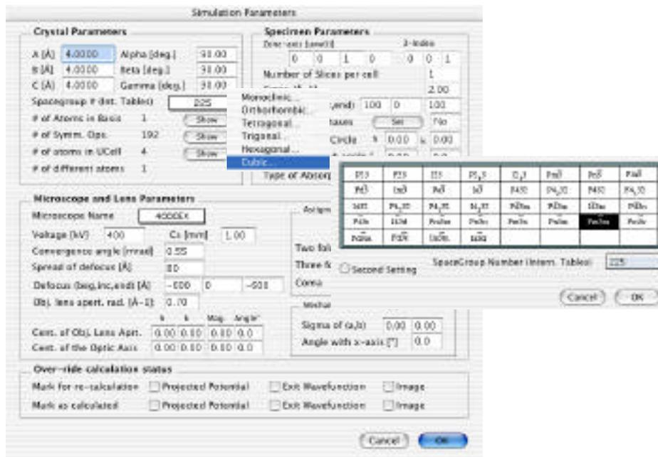
The input also allows for choosing the second setting for a specific spacegroup if one exists. If no space group is required, one should use the space group P1 (1), in which case the only symmetry operator is x,y,z. Additional symmetry operators can be entered by opening the dialog displaying the symmetry operators.
