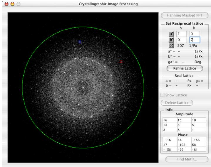
reflections used in the lattice refinement and information extraction can be limited by the circular aperture tool. Once the lattice reflections have been marked, the next action is to invoke the command “Refine Lattice”.
