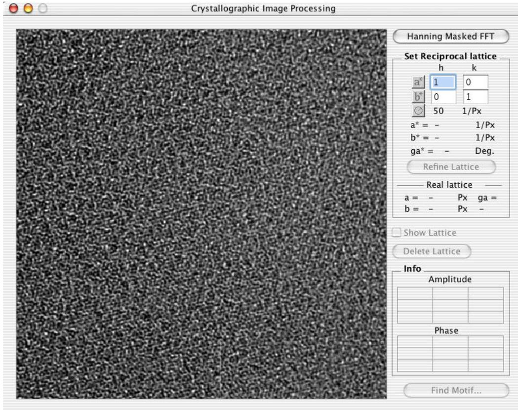
Fourier transform need to be calculated. Once the Fourier transform has been calculated, the reciprocal space lattice needs to be set using the  $a^*$  and  $b^*$  tools and clicking on two consecutive
