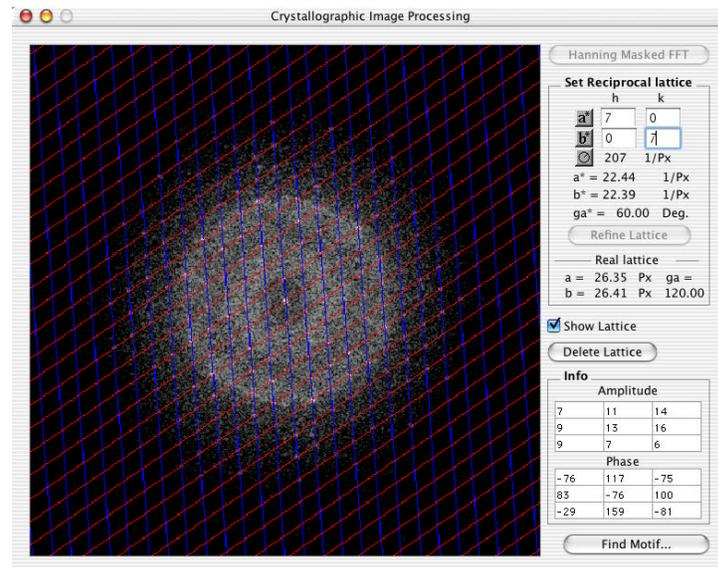
After the lattice has been refined, click on “Find Motif”. This will extract all the phases and amplitudes from the Fourier transform at the lattice points and one can test for possible symmetries of the motif.
