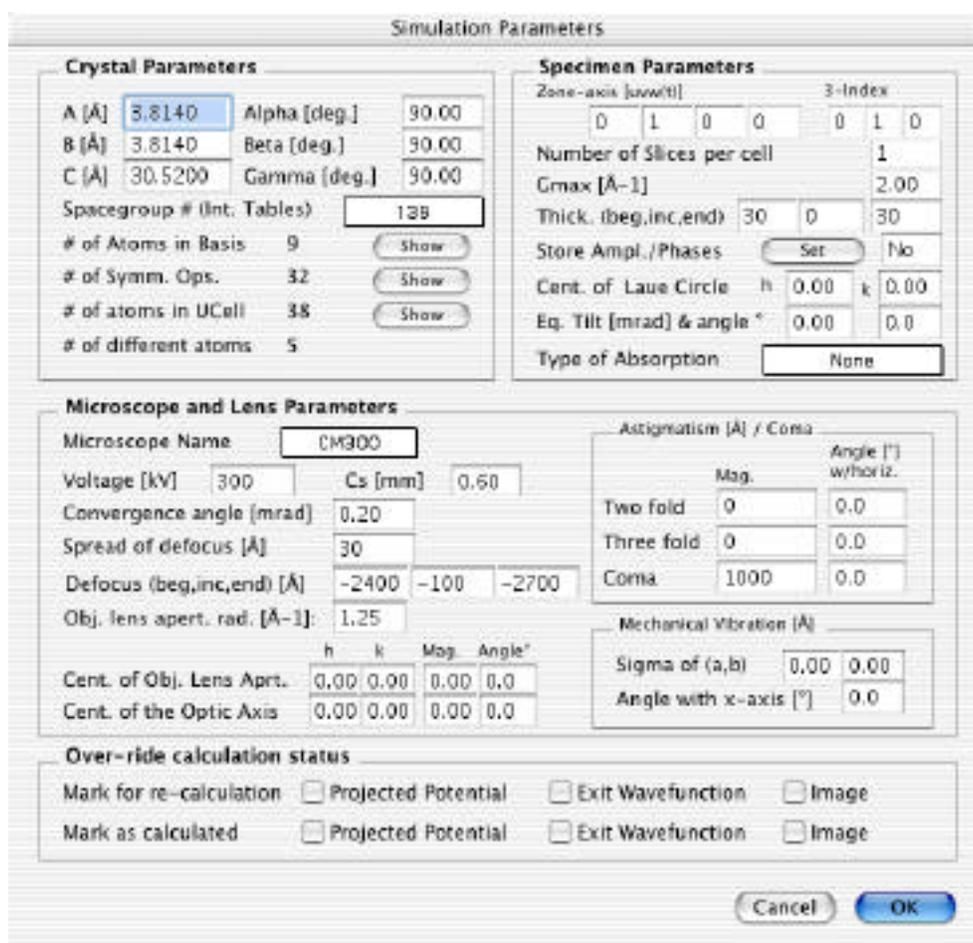
New... command in the FILE menu. The parameters can be changed as to bring about a new simulation.
