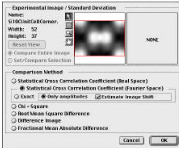
This calculates the CCC based only on the Fourier amplitudes and (optionally) the program will try to estimate the shift between the experimental and the calculated image. This can be very useful for aligning images and to compare images when the origin of the experimental image is not known. The numbers given are the shift of the origin that should be attempted to be made on the experimental image before the experimental data is
