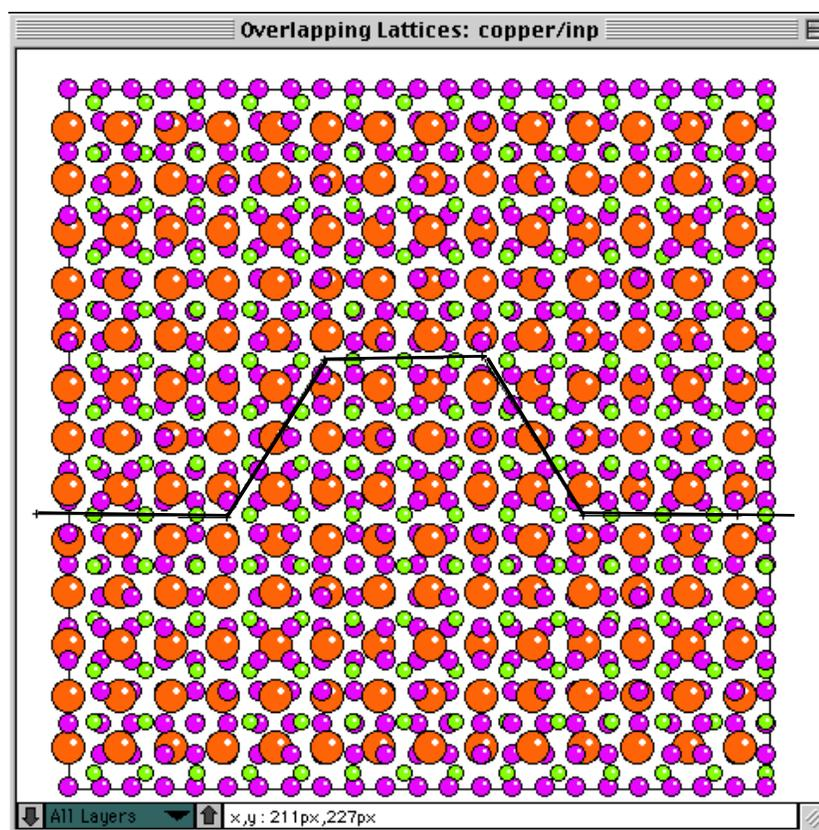
When the last point is defined (to the right of the drawn region), the defined interface will be automatically drawn. Atoms can be individually moved or deleted to fine tune the interface before a unit cell is selected with the Unit Cell Tool.
