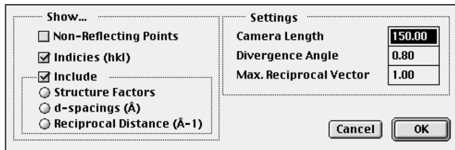
The maximum reciprocal lattice vector is set through the dialog together with options for labelling the pattern. The options are i) indexing the pattern (hkl), ii) showing structure factors, iii) showing d-spacings and iv) showing length of reciprocal lattice vectors. If the “Show non-reflecting points” is checked, the program will also display points in the reciprocal lattice that are in non-reflecting positions.
