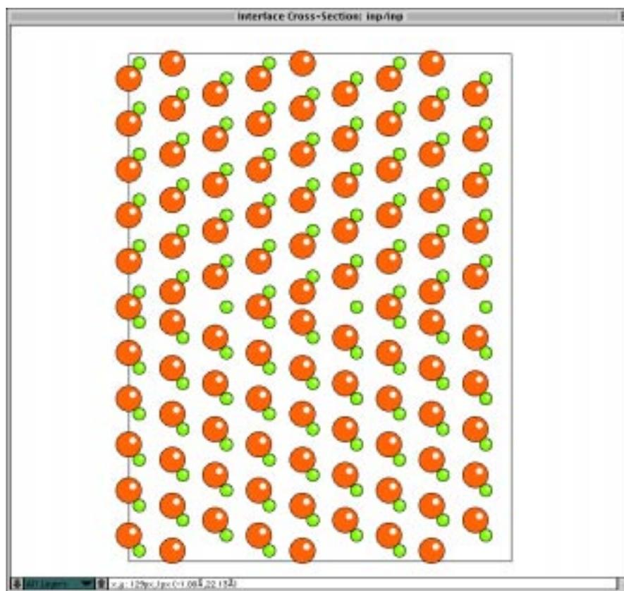
If you now want to define a unit cell, just use the “Define Unit Cell” Tool and mark the Origin, A and B. At this point you will have a double set of atoms at the interface plane, because both
