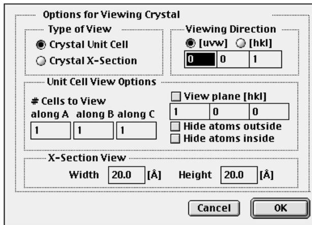
The field of view and the specification of the zone axis are only associated with drawing a crystal cross-section and the zone-axis does not have an effect when displaying a single unit cell. When the display of a single unit cell is specified, the unit cell is always initially drawn in the [001] orientation. The crystal can be rotated into an arbitrary orientation with the Rotate Tool.
