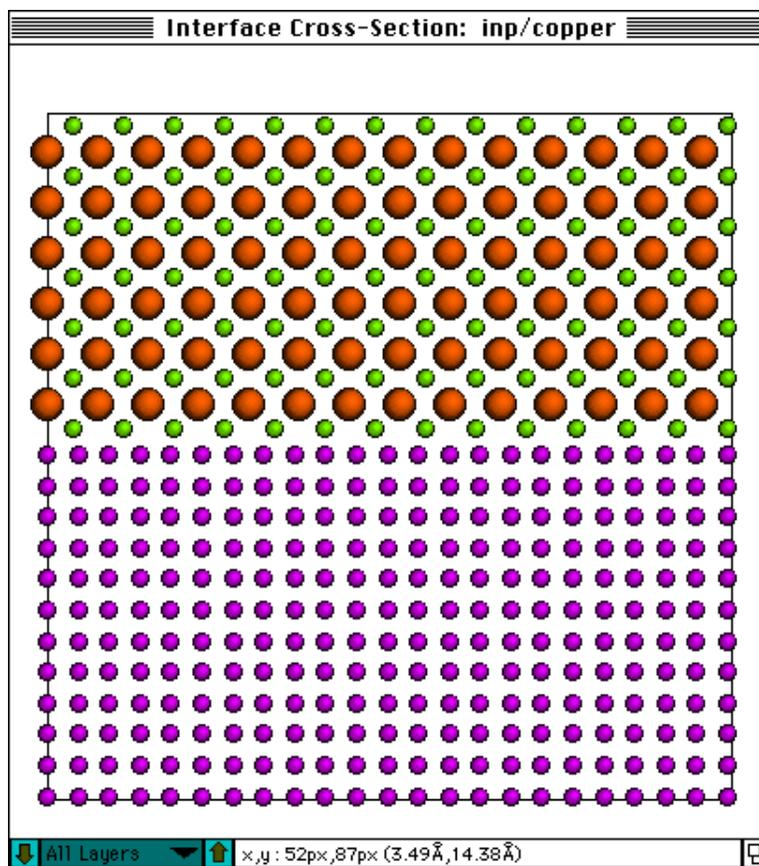
This window is used for all drawing of unit cells etc. When drawing a cross-section, the layer control at the bottom of the window can be used to display only atoms in specific layers. The control is a pop-up menu, displaying the various heights in
