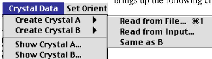
If the data is read from file, the normal Apple file-dialog appears, allowing the user to select an input file. If the **Option** key is held down when selecting "Read from File..." the program allows the user to choose an EMS file to be read in. No check on the filename is performed and the file must be a valid supercell EMS file.
